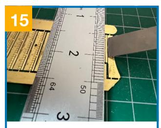
Use a metal ruler and a flat scalpel blade, lift each beam 90 degrees.
