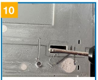
To provide finer adjustment of the light output location, you may want to use the Rotary tool to make a wider hole.
