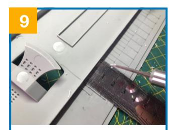
Using the 1mm Scribing tool and a metal ruler, cut channel along your marked lines
