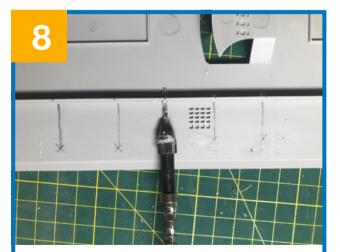
Drill through the LED strip wall with a 1mm drill bitt.
