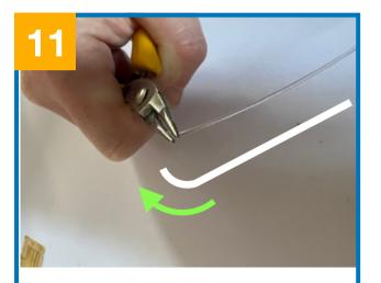
Using Round Nose Model Pliers, create a 90 degree bend at the end of the Fibre strand.
