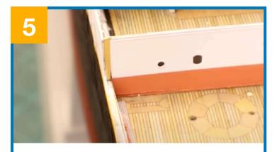
If you are using the PE Hull plating; you will need to fill this 2mm gap at either end. Use off-cuts of brass or styrene.
